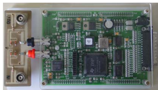
FIGURE. 2 DSP TMS320C31 MODIFIED CARD.
