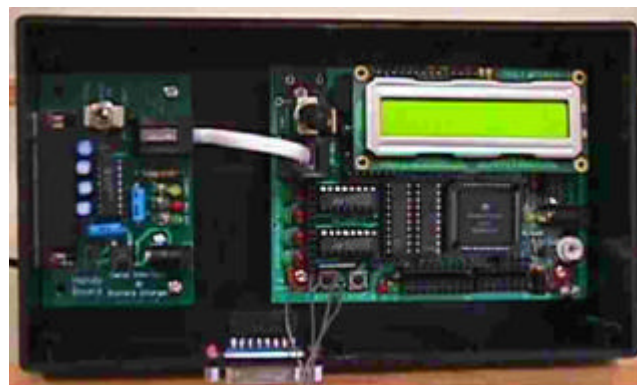
FIGURE. 1 HANDYBOARD DEVELOPMENT SYSTEM.
