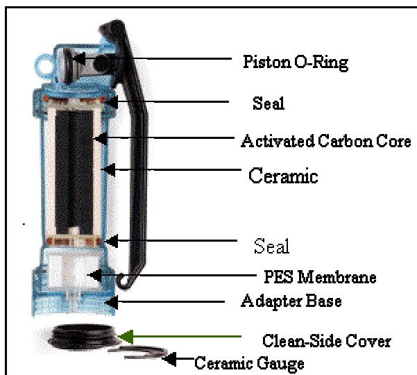
Figure 1: Components of a MSR filter
