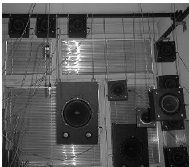
FIGURE 2 MEASUREMENT MICROPHONES AND LOUD-SPEAKERS FOR THE 3-DIMENSIONAL ZONE OF QUIET GENERATION.
