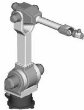
FIGURE 2 ANGULAR ROBOT WITH 6 DOF
