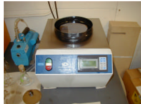
FIGURE. 1 SCS P6708 SPIN COATER WITH SILICON WAFER
