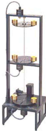
Figure 4: Three degree-of-Freedom torsional plant at UNF.
