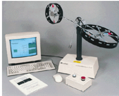
Figure 2: Twin rotor plant at CUAS.
