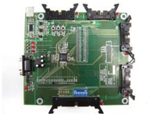
Figure 02 – Base Module developed for the BSPS-DM.
