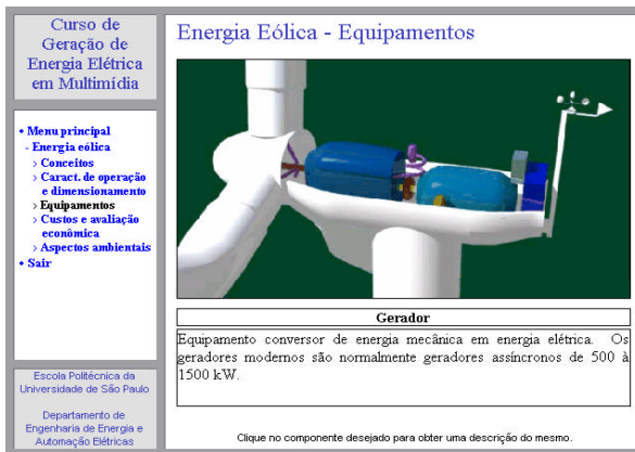
Figure 3- Aeolic Energy equipment screen.
